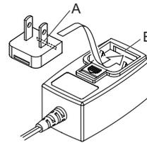
Push the AC plug in from above while pulling the C section.
