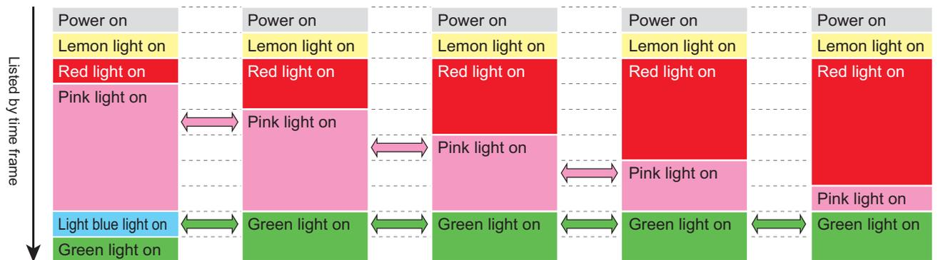
\* Depending on the installation environment and radio wave conditions, the lighting and flashing status of the indicator may not transition as shown in the figure.
