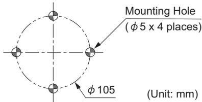
\* Screws (M4 or nominal diameter 4) to secure the bracket are not included. Please provide your own. (bracket thickness: 7 mm)
