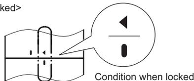
Align and fit the positioning marks and turn clockwise to lock.
