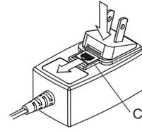
\*The plug in the diagram indicates UL. Work on the other AC plugs in the same manner.
