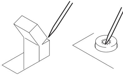
Switches are deformed or buttons are damaged
