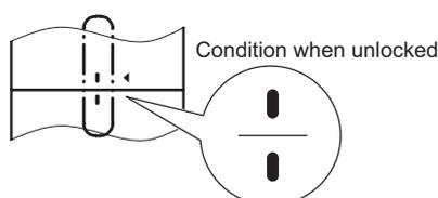
While holding the adjacent lower unit, turn the unit to be removed counterclockwise to unlock it and lift it up.
