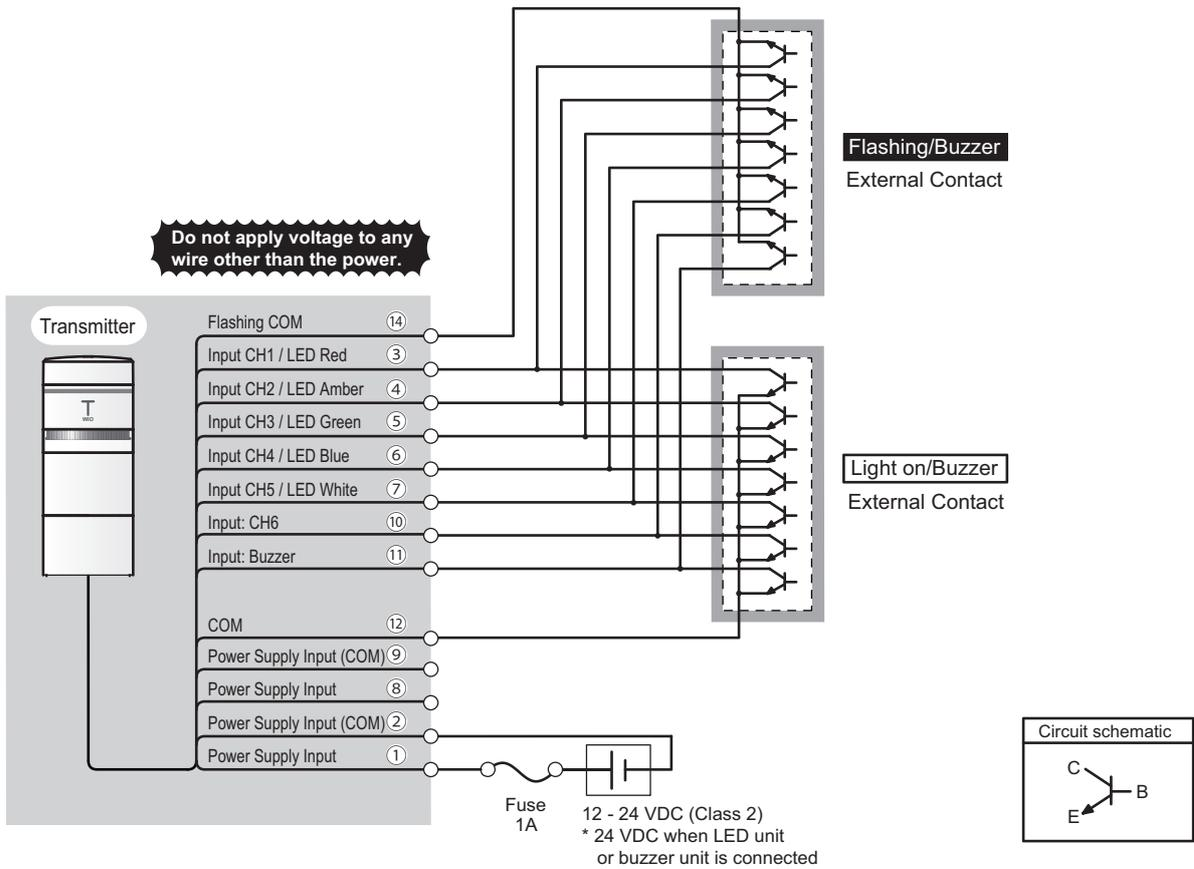
● External contact classification: PLC (PNP transistor)
