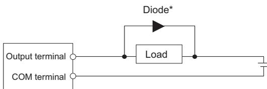
\*Reverse withstand voltage: 3 times or more than the load voltage
