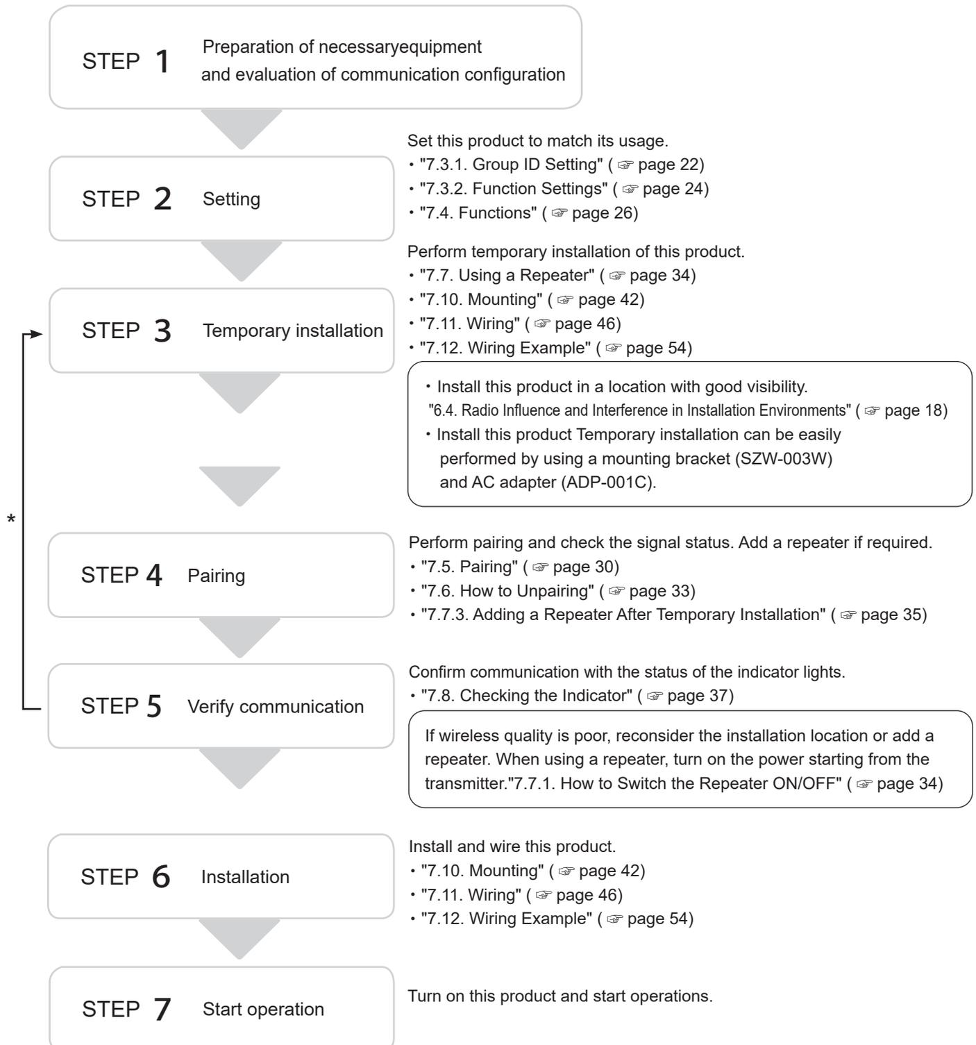
\* If the communication check results show that the signal is poor and the installation location needs to be reconsidered, start over from STEP 3.
