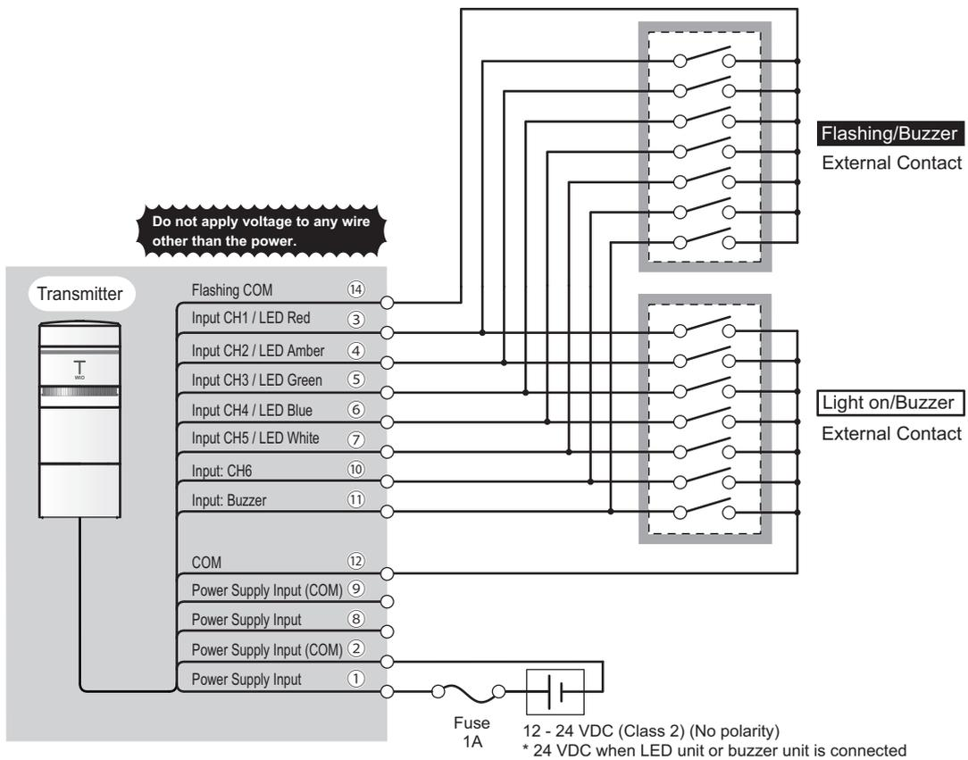
● External contact classification: PLC (NPN transistor)
