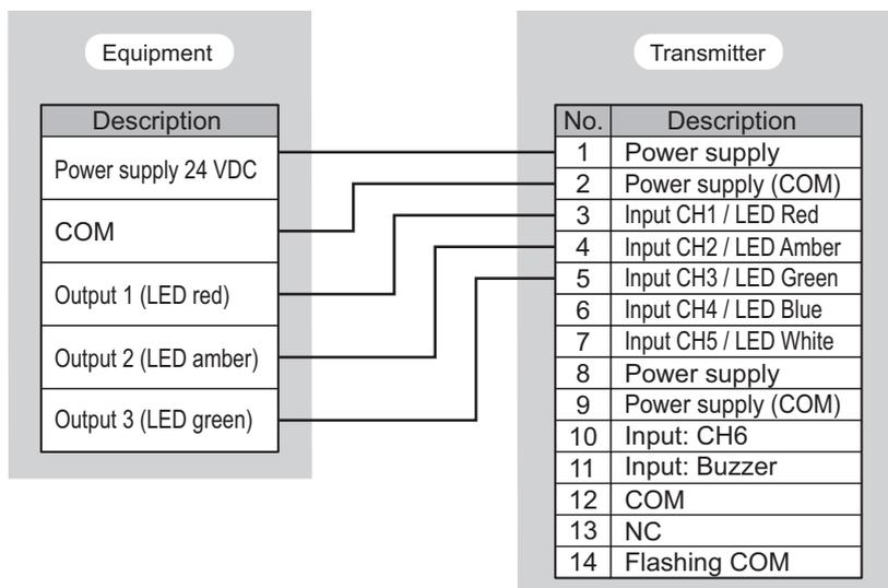
Wiring of repeater/receiver and alarm
